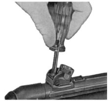
Loosening the clamping screw
